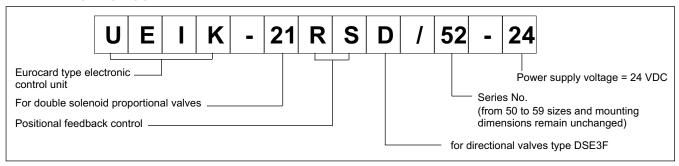
The UEIK-21RS card is an electronic control unit Eurocard type for closed loop control of double solenoid proportional valves with positional feedback control.
