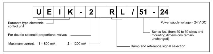
The UEIK-2\*RL card is an electronic control unit in Eurocard format for open loop control of double solenoid proportional valves, with selection in sequence of four different reference and ramp time regulation signals.
