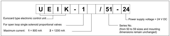
The UEIK-1\* card is an electronic control unit Eurocard type for open loop single solenoid proportional valves.
