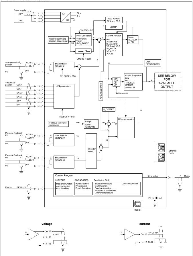
**NOTE**: If the card is configured as simple positioning control without pressure limitation then the output value is calculated just from the output of the position controller (CS) instead of apply MIN and MAX parameters. MIN/MAX are selected by the PQInverse bit (Fieldbus).
